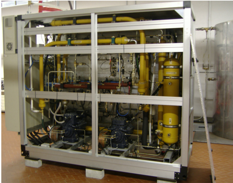
Figure 4.14 - Picture of the refrigeration cycle with CO 2 .
