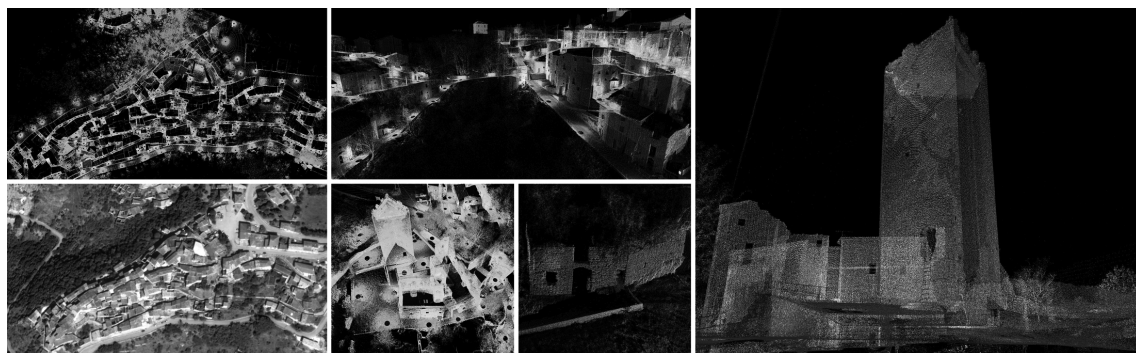
Snapshots of point clouds views of the laser scanner survey of the Acciano's center and Beffi's castle.
