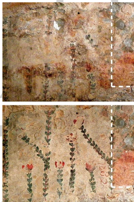
Figure 2. Application of the EAPC o/w nanostructured fluid on wall paintings from the Annunciation Basilica in Nazareth (Israel). Top: Before restoration. The alteration of the surface by aged coatings is evident. Bottom: After restoration. In the dashed box, an area is highlighted where the polymer coating has been left untreated as a reference for the evaluation of the cleaning result. Reproduced with permission from Ref 13. Copyright 2012 American Chemical Society.
