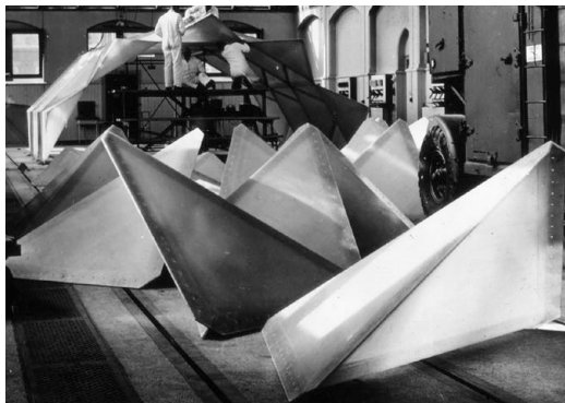
6. Pezzi piramidali in poliestere rinforzato con, in secondo piano, la struttura a volta risultante, assemblata allo Space Structures Research Centre. © Space Structures Research Centre, University of Surrey.
