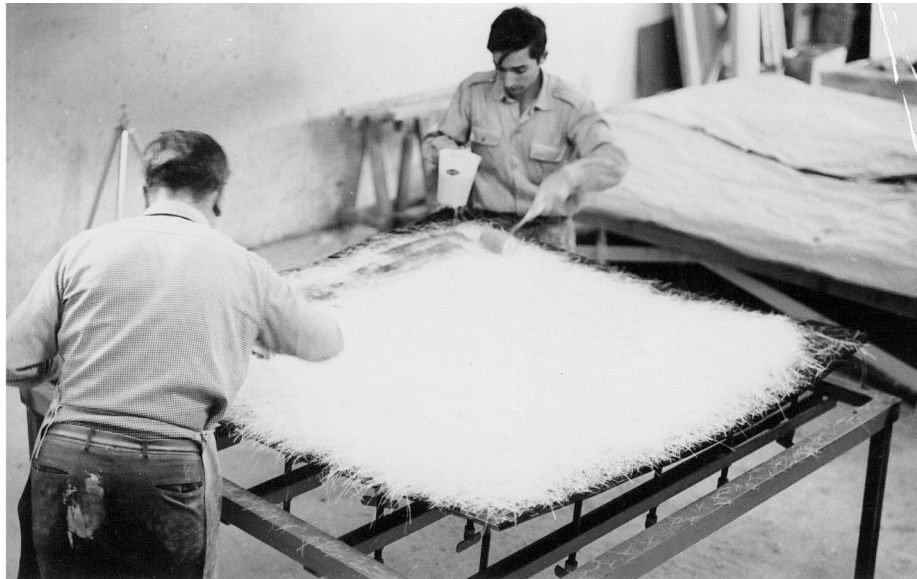
Figure 5: The flexible sheet of rubber on which the pieces of the structure are formed.
