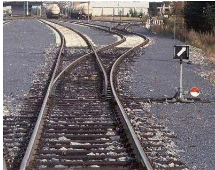
Figure 1.9: A simple 2-way switch: source wikipedia
