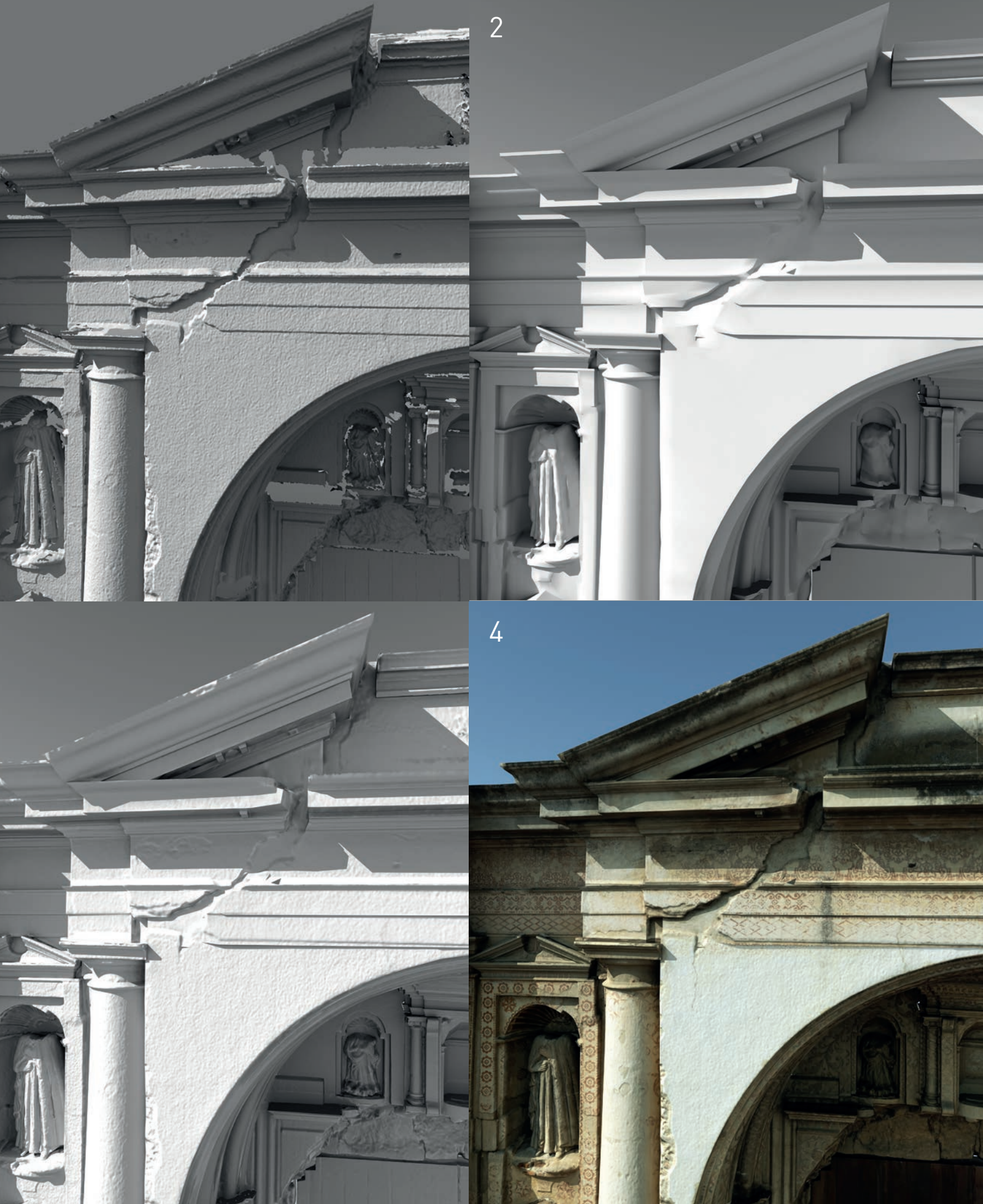
1. Modello high-poly; 2. Modello low-poly; 3. Modello low-poly con Normal Map applicata; 4. Modello low-poly con Normal Map e Diffuse Color Map.
