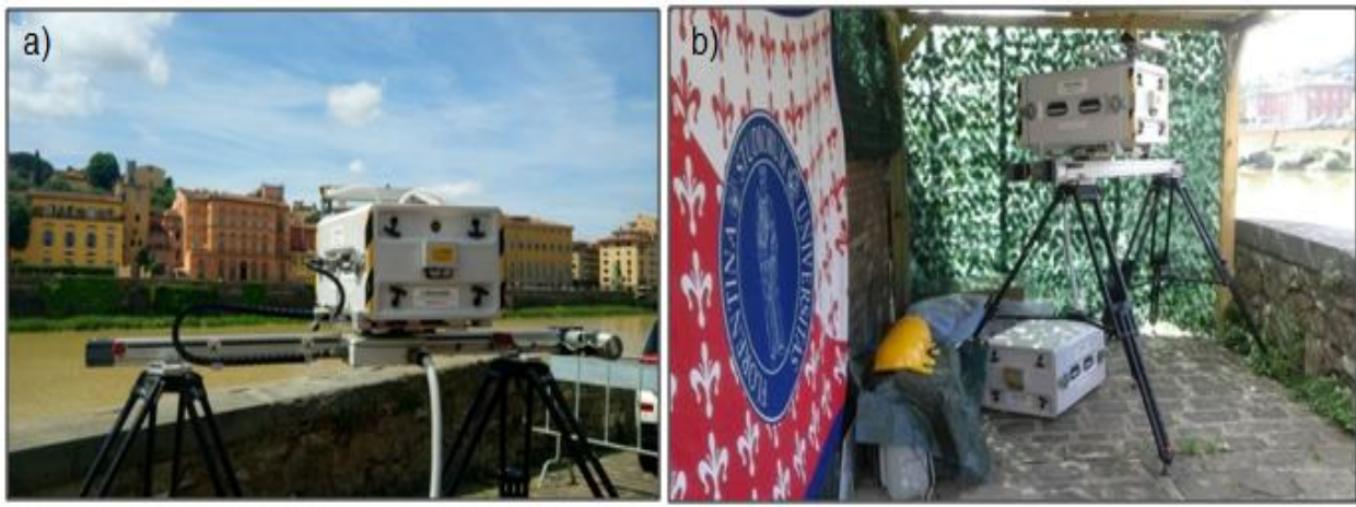
Figure 42. a) GBIInSAR instrumentation positioned in the riverbanks opposite to Lungarno Torrigiani, and b) wooden cabin built to protect the GBIInSAR.
