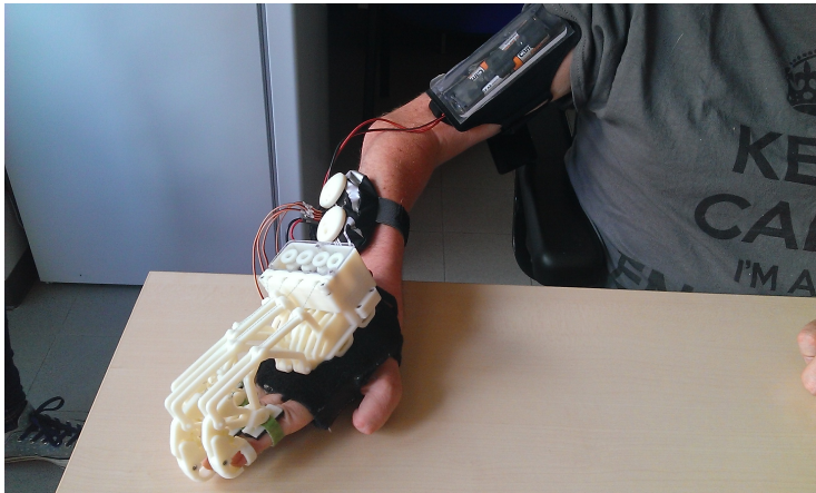
Figure 4.1: The first version of the hand exoskeleton prototype worn by a patient.
