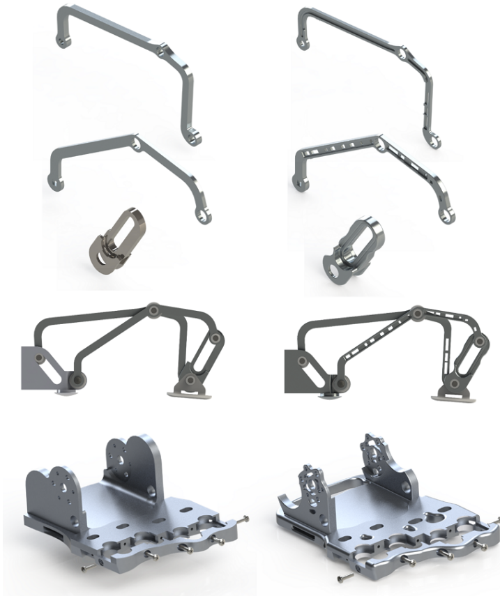
Figure 5.9: Reconstruction process results of the hand exoskeleton mechanism components. Component B and the back frame are represented in section view to highlight the internal holes.
