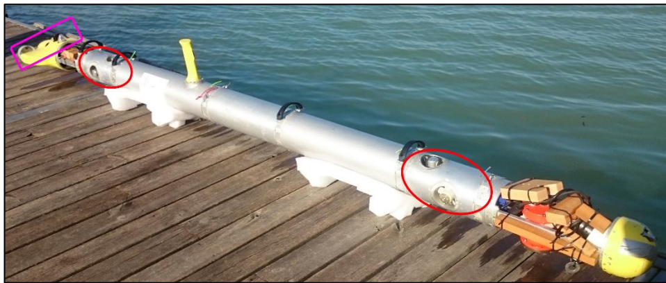
Figure 3.3: Marta AUV thrusters position: tunnelled thrusters (4) in circle red and stern thrusters (2) in circle purple.
