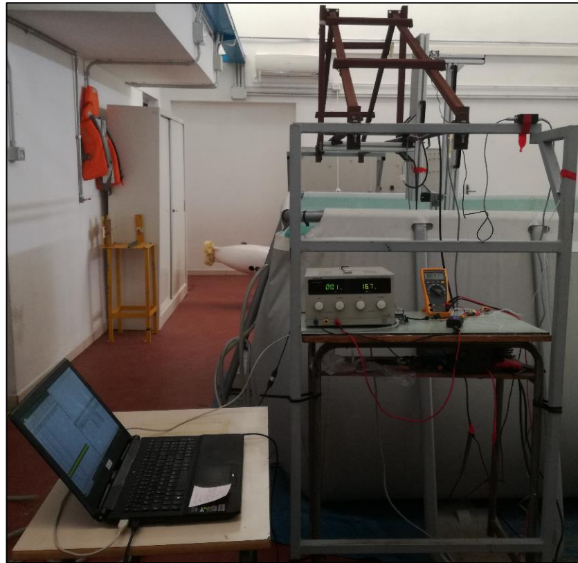
Figure 3.24: The whole new thruster measurement chain, during the last thruster test.
