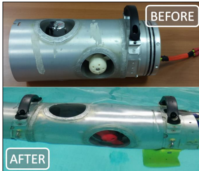
Figure 3.6: Comparison between the old and the new version of MARTA tunneled thrusters.
