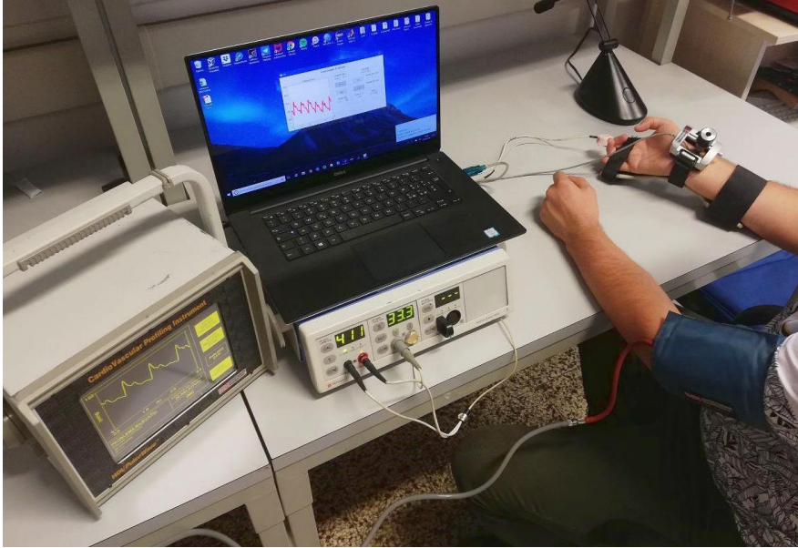
Figure 7.1: Picture of the experimental setup, showing the CR-2000 CardioVascular Profiling system (left) and the Periflux LDF system (right), the positioning of their respective proprietary sensors, and the blood pressure cuff needed for calibrating the radial pressure waveforms.
