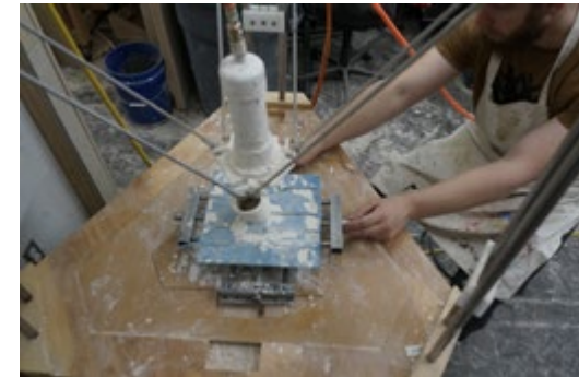
02 Craftsperson using manual x,y-axis controls to improvise ceramic form. Photo by author
