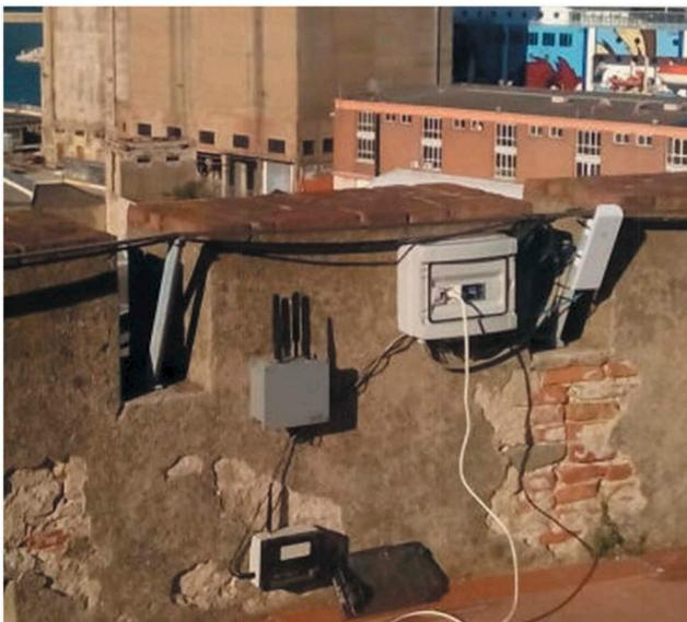
**Figure 2.** View of the gateway (installed on the tower case study).
