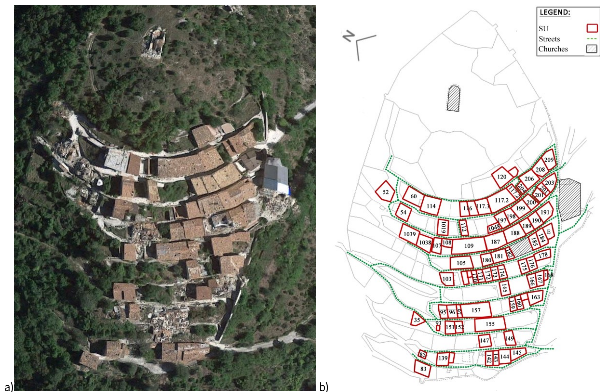
Figure 3.5: View of Campi Alto di Norcia after the 2016 earthquakes (a); Identification of Structural Units, highlighted in red and identified with different IDs, within Campi Alto di Norcia (b).
