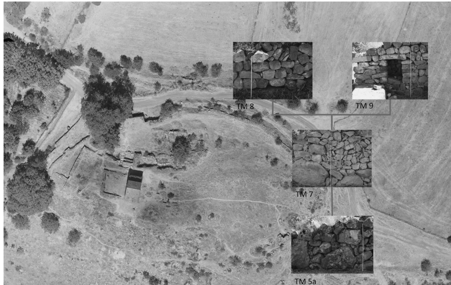
Figure 2.5. Stratigraphy of masonry types in unsquared stones from the architectural complex of Zorats' church
