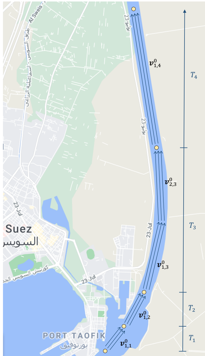
Figure 4.8: Sequence of OU velocities and time intervals characterizing the nominal dynamic behavior of the Ever Given inside the Suez Canal given the available sequence of AIS contacts.
