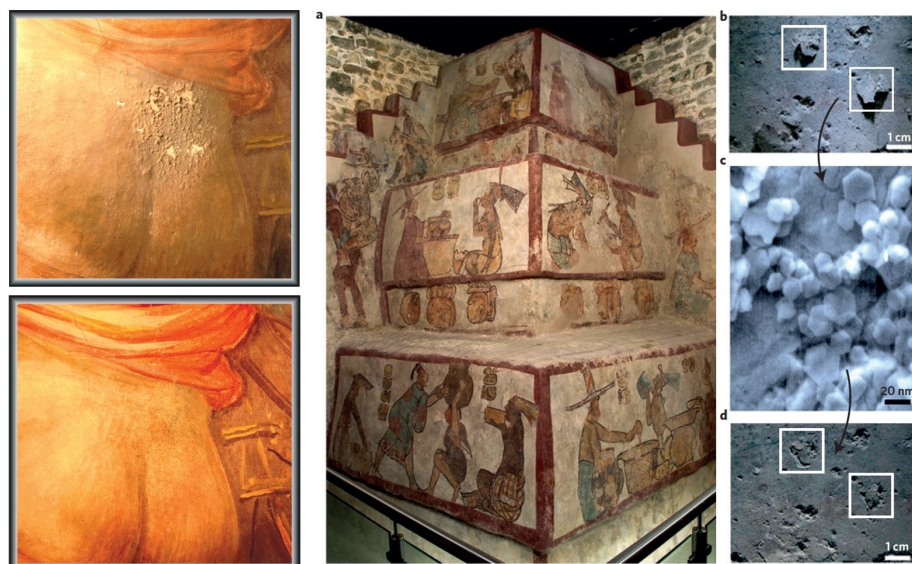
Figure 1. Left: Application of \text{Ca}(\text{OH})_2 nanoparticles for the consolidation of Renaissance wall paintings in Florence Cathedral. Top: before and bottom: after restoration. Reproduced with permission from ref. [15]. Copyright: 2001, American Chemical Society. Center and right: Mayan wall paintings in the United Nations Educational, Scientific and Cultural Organization world heritage site of Calakmul (Mexico). a) Photograph of the wall paintings after restoration with \text{Ca}(\text{OH})_2 nanoparticle dispersions. b) Grazing visible light image showing the detaching paint flakes before the application of nanoparticles. c) Scanning electron microscopy micrograph of the \text{Ca}(\text{OH})_2 nanoparticles (hexagonal platelets) that were applied to the degraded painted surface. d) Grazing visible light image showing re-attached and re-adhered paint flakes after the application of nanoparticles. Panels a, b, and d reproduced with permission from ref. [13c]. Copyright: 2014, The Royal Society of Chemistry. Panel c reproduced with permission from ref. [12]. Copyright: 2015, Macmillan Publishers Limited.
