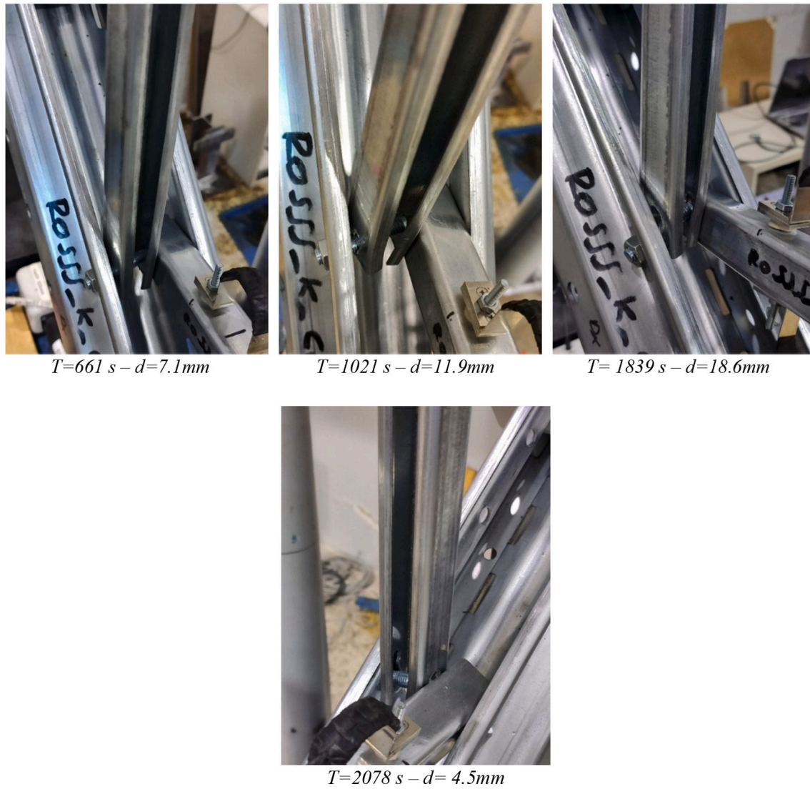
Fig. 15. Test c2M8-dhB - Specimen deformation for different displacement steps.
