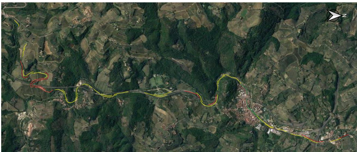
Figure 5.30 – HFESs colored based on the Total HFS result: HFS < 40\% (red), 40\% \leq HFS \leq 60\% (yellow), HFS > 60\% (green)
