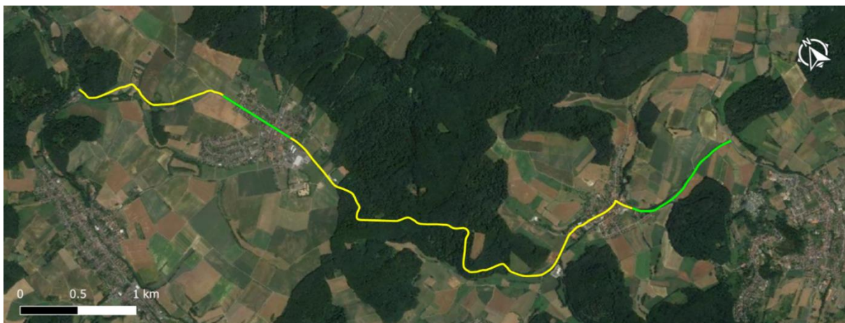
Appendix Figure 20 – L3408, stretches with the same CCR on satellite image (red= high CCR, yellow = medium CCR, green = low CCR)
