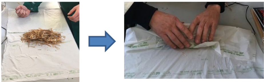
Figure 2. Current manual rolling process for obtaining the straw-bioplactic cylinders
