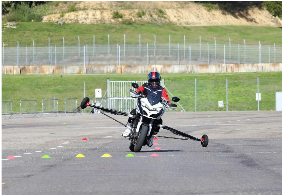
Figure 4 – Test vehicle (Ducati Multistrada 1260S) with extension arms during lane-change maneuver
