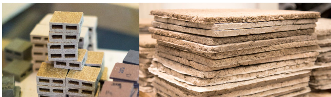
Fig. 2. Extruded wood-plastic composites from recycled raw materials (LUT University and Linnaeus University).
