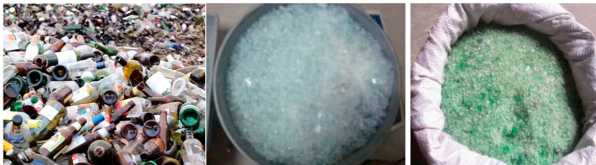
Fig. 4. Glass waste converted into coarse aggregates and fine glass powder (part of the photo is taken from Ref. [84]).
