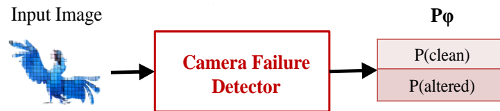
c) Structure of a Camera Failure Detector (CFD)
