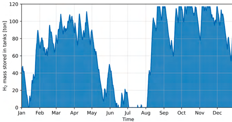
Fig. 6. Trend of the H 2 volume stored in tank storage in a configuration equipped with a 117 tons of hydrogen storage capacity.
