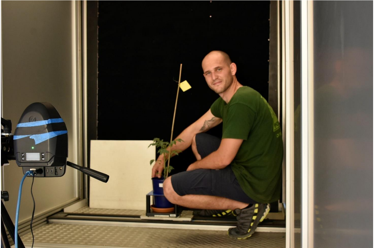
Figure 2. Hyperspectral acquisition process on tomato plant. The white Lambertian surface reference target at 75% of reflectance is the white panel on the plant's left.
