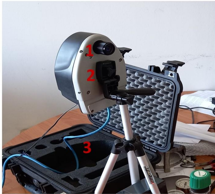
Figure 2. Hyperspectral camera HSC-2. Further information can be found at the link of the instrument web page https://senop.fi/product/hsc-2-hyperspectral-camera-450-800nm/ .
