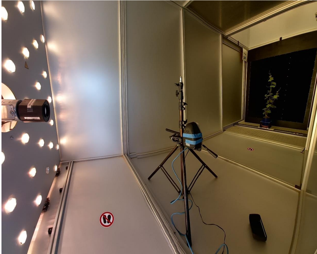
Figure 4. The acquisition chamber was used in the experiment. In the image are visible the light source, the HSC-2 and a vegetation target in the background.
