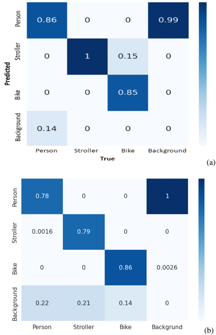
Fig 5. confusion Matrixes on the validation dataset of CAM52: (a) YOLO-CAM52-MODEL, (b) FRCNN-CAM52-MODEL
