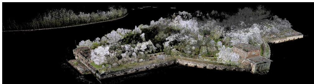
Fig. 6- 3D colorimetric point cloud of the fort
