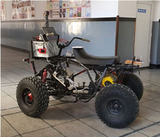
Fig. 3 The hardware assembly of the LiDAR mapping system mounted on the electric ATV
