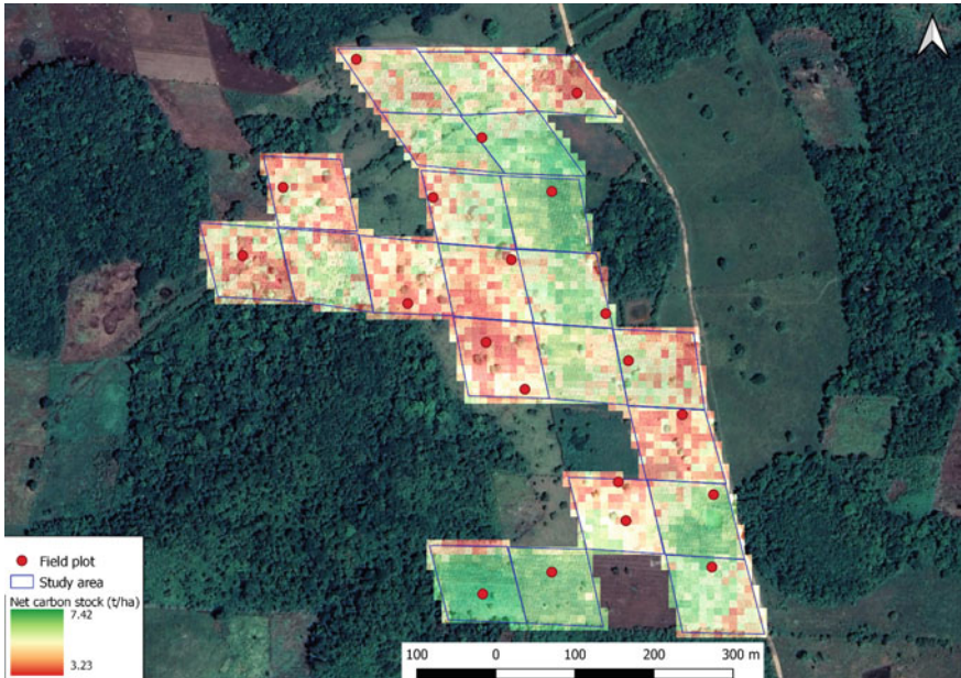
Fig. 4 Net equivalent CO 2 stock map generated with RF model. In blue the study area grid, while red dots represent the ground samples
