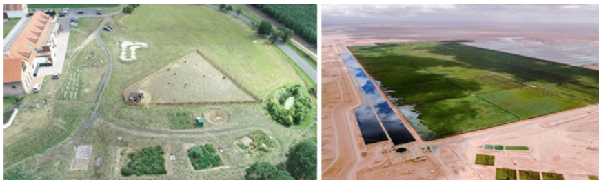
Fig. 1 Left: a constructed wetland system in the Czech Republic for wastewater treatment and reuse. Right: a constructed wetland system in Oman for oily water treatment reuse
