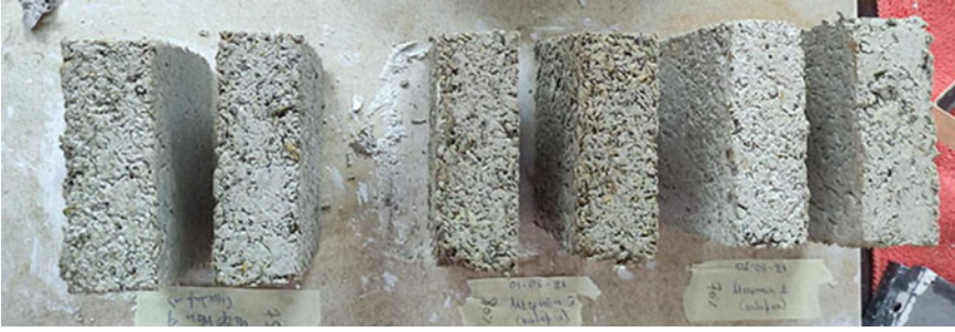
Fig. 2 Images of the samples AD3-LP2, AD3-LP4 and AD4-G8 dried in ventilated and dry conditions
