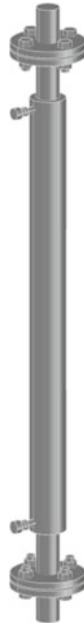
Fig. 1 Schematic illustration of the double tube reactor with the in- and outlet fittings for the thermal fluid
