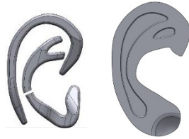
Figure 21 - Example of CAD models of the surgical guides created by simplifying the original anatomy.
