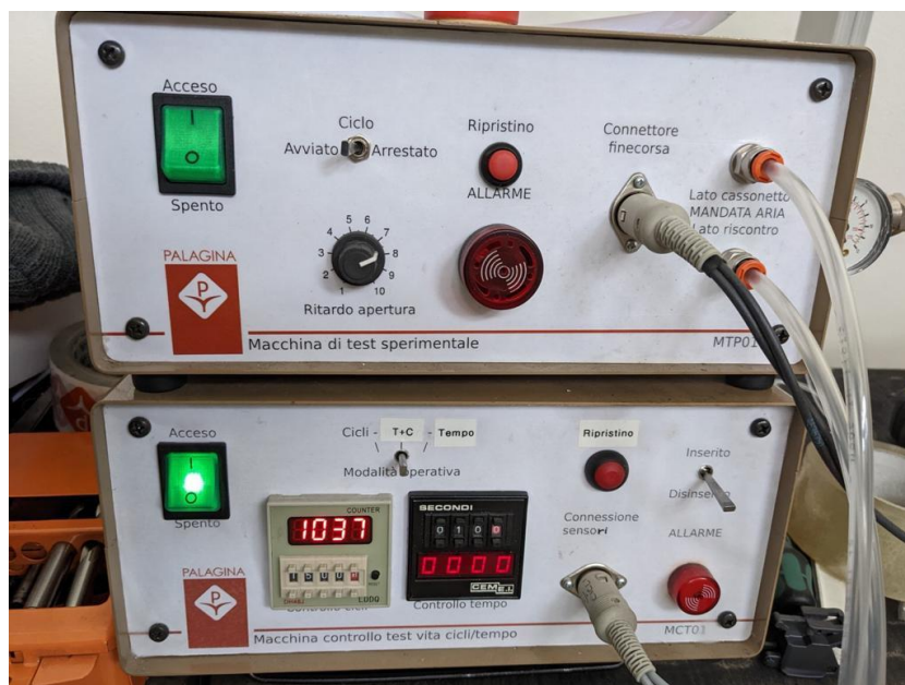
Figure 4.8 – Electronic control unit for the setting of life tests.
