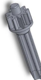
Figure 5.10 – First gear co-axial with the tube.
