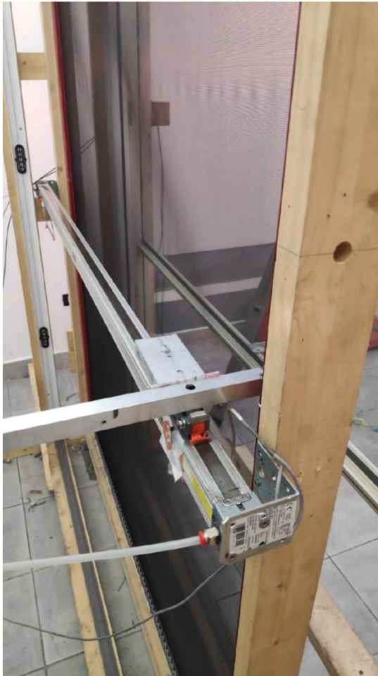
Figure 4.7 – Pneumatic piston employed for the moving of the handlebar during life tests.
