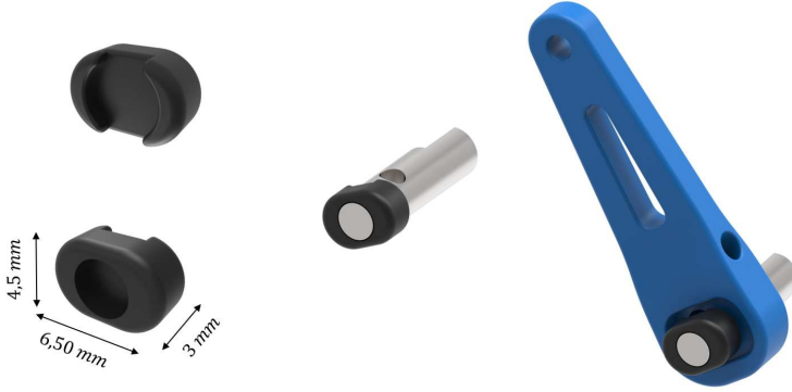
Figure 3.18: The housing designed for the magnet to be installed in the shaft: on the left, its front and back views with indications of overall sizes; on the centre, the magnet with its housing arranged on the shaft, and on the right, a view of the actuated joint of Link 1.
