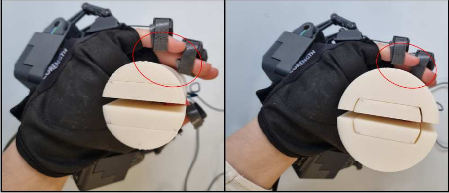
Figure 4.21: Fingers not in contact in grasping the 50-mm cylinder, on the left, and the 75-mm one, on the right.
