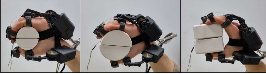
Figure 4.10: The grasping tasks: a view of the 50-mm cylinder, 75-mm cylinder, and 75-mm cube grasps.
