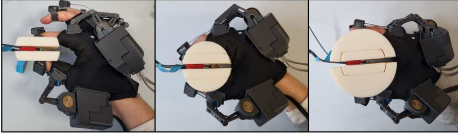
Figure 4.20: The gripping tasks administered: from the left to the right, the pinch task, the 50-mm and 75-mm cylinder grasp, in which the improved adherence of the new exoskeleton embodiment is visible.
