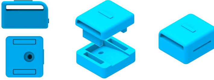
Figure 3.21: Views of the distal phalanx EE: on the left, a side and bottom views, on the centre, an axonometric view of the two components, and on the right, the definitive distal phalanx EE.
