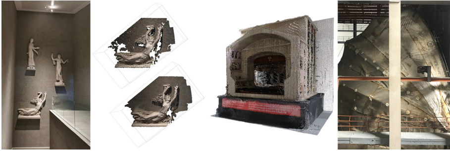
Fig. 4. 3D laser-scanner and SfM photogrammetric survey of the wooden model and statues.
