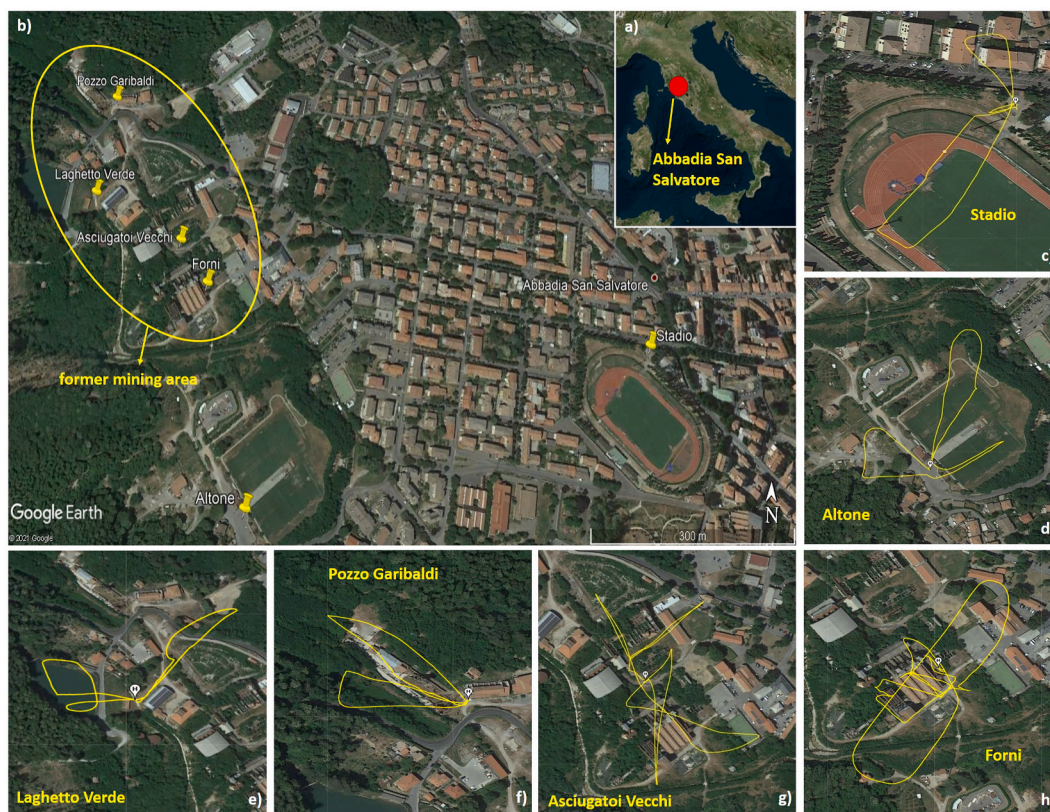
Fig. 1. Location of Abbadia San Salvatore (Mt. Amiata, central Italy) (a) and the former Hg mining area (b). The flight routes carried out by the UAV-Lumex pair at the selected six sites are also reported: “Stadio” (c), “Altone” (d), “Laghetto Verde” (e), “Pozzo Garibaldi” (f), “Asciugatoi Vecchi” (g) and “Forni” (h). See text for additional information.
