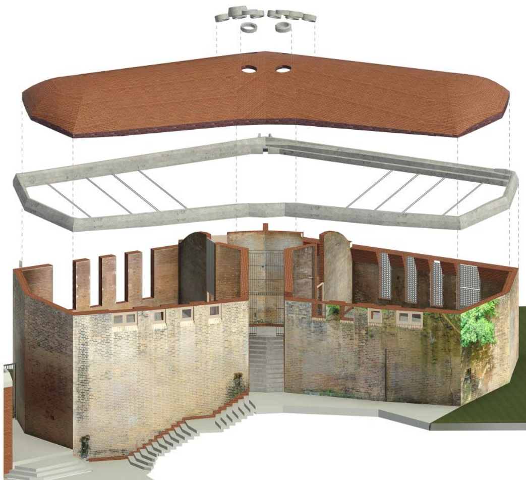
Fig. 5. 3D exploded view of block 5 (elaborated by Bongini, A.)
