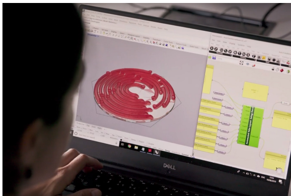
Figure 13. Case study ADAM - Acoustics by parametric Design and Additive Manufacturing. The product design phase uses computational design models and associated software such as Rhinoceros and Grasshopper (Source: video frame of the project presentation made by the research team, [72]).
