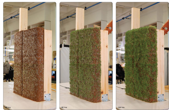
Figure 12. Case study Living soil walls (CS.11). Germination stages of Living Soil Wall at 48, 96, 144 hours after printing (Source: DeZeen, [64]).
