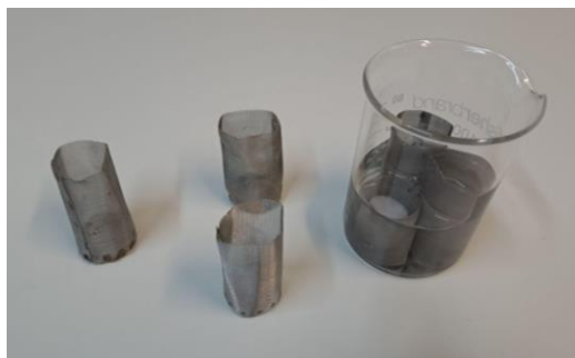
Figure 33. An example of how the purpose-built metallic cages look like and how a swelling degree test was conducted.
