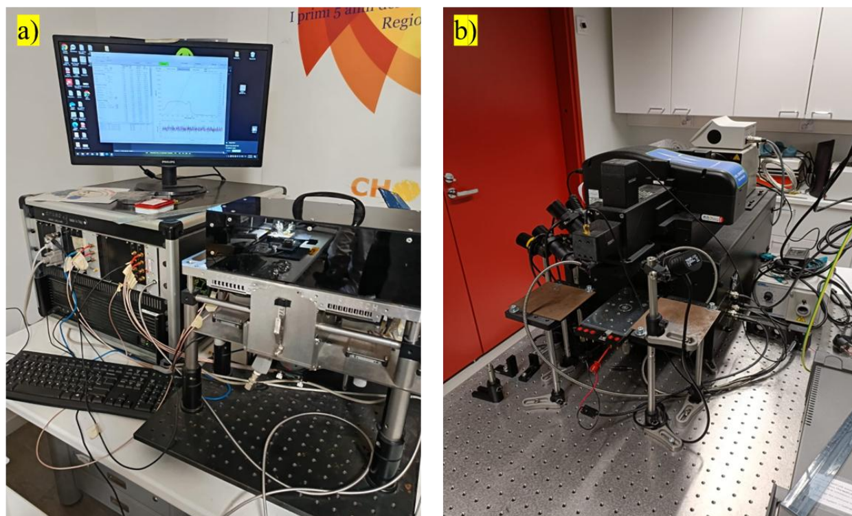
Figure 3.8. a) Optical power density-based measurement system (Arkeo-Cicci research s.r.l.) in CHOSE, Italy, b) EQE measurement system (QuantX-300, Newport) in the University of Tampere, Finland.
