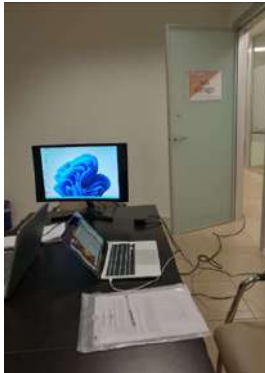
((a)) The observation room: laptop for the moderator; laptop for the observer; printed task list and supportive documentation; external monitor, connected via an HDMI cable to the test workstation [31]
