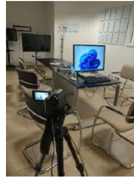
((c)) The test room for mouse/keyboard modality: traditional display, mouse and keyboard placed on a large desk; comfortable chair; workstation with tested software installed, connected through an HDMI cable with an external display; smartphone, placed on support with angular regulation; camera placed on a tripod.
