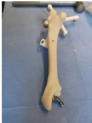
((b)) Metal stem inserted in the 3D printed model
