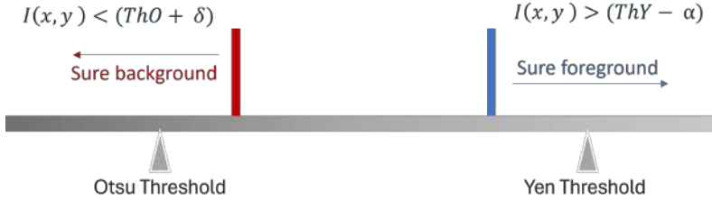
Figure 6.2: Thresholding scheme proposed to initialize graph cut
