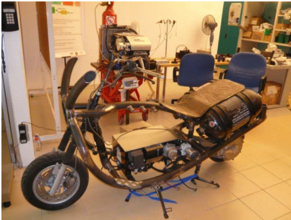
Figure 2.10: Pios Fuel Cell Motorcycle prototype frame [300]
