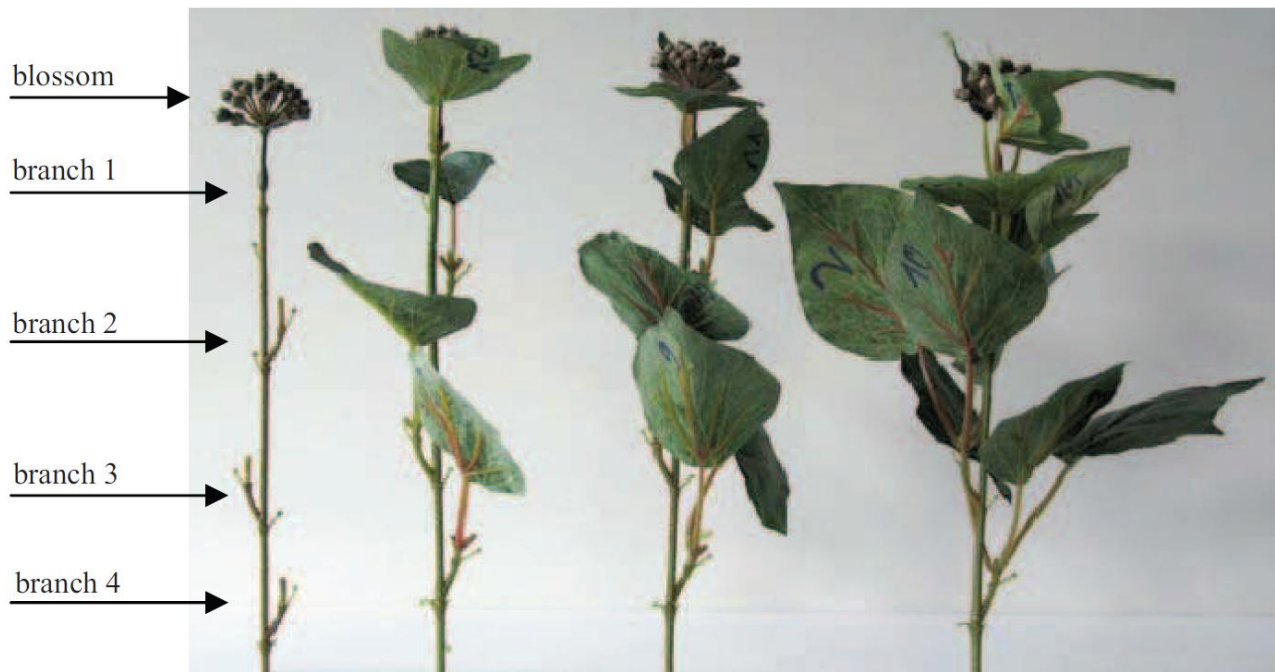
Figure S2. 1 - Artificial poplar at different stages of foliation (from left to right: stem with blossom, stem with branches carrying one leaf, stem with branches carrying two leaves, and stem with branches and three leaves, respectively. (Schoneboom & Aberle, 2009)
