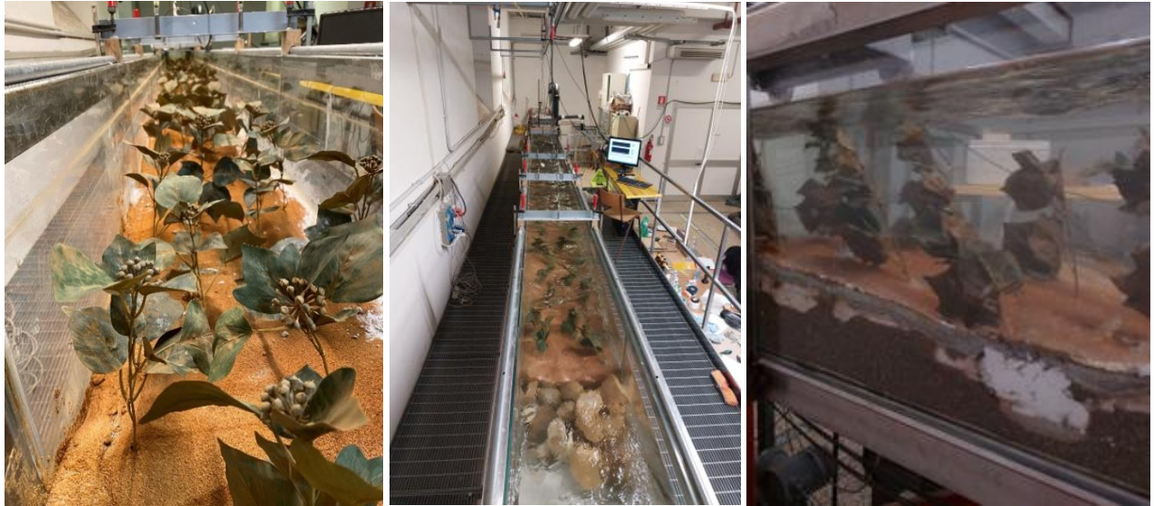
Figure S2. 2 - Views of the experimental flume setup with artificial riparian vegetation. (a) Photograph of the central portion of the hydraulic flume showing artificial Populus alba plants positioned over the fixed dune bed. In this configuration (XBCD), the lowest foliage layer (A) has been removed, while branches B, C, and D are present. (b) Top view of the 10.5 m recirculating flume during a test run, showing the vegetated section installed over the fixed dune bed. Flow direction is from bottom to upper part; upstream and downstream sections are stabilized with gravel layers. (c) Lateral view of the vegetated section under quasi-steady flow conditions (mean depth \approx 23 cm), showing artificial Populus alba plants interacting with the current. The dune-shaped bed is made of painted polystyrene and covered with sediment.
