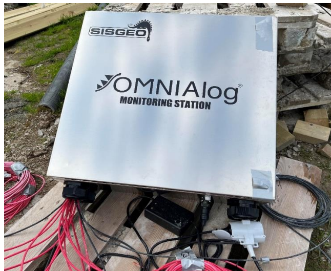
Figure 3.17: Sensors connected to the Omnialog datalogger.
