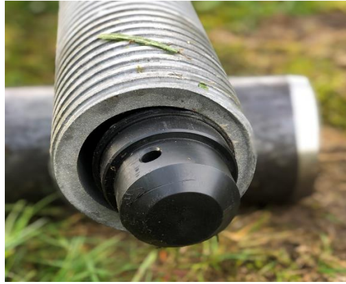
Figure 3.14: Coaxial pipe in hollow bar.
