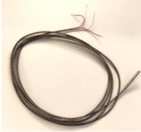
Figure 3.5: Micropile temperature sensor.
