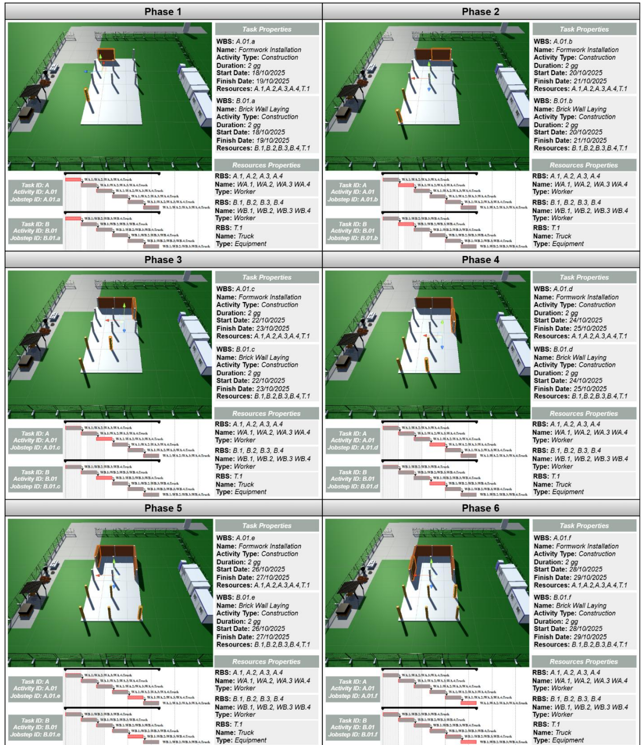
Figure 21 - Activity Sequence and Task Properties Visualization of the Test Model 4D BIM
