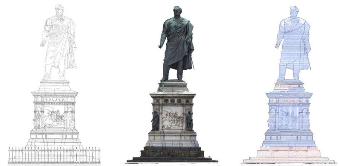
Fig. 2 - Florence, Monument to Manfredo Fanti, geometric and dimensional data representation, photoplan and deterioration analysis (Graphic processing by P. Bordoni, A.L. Petracci).
