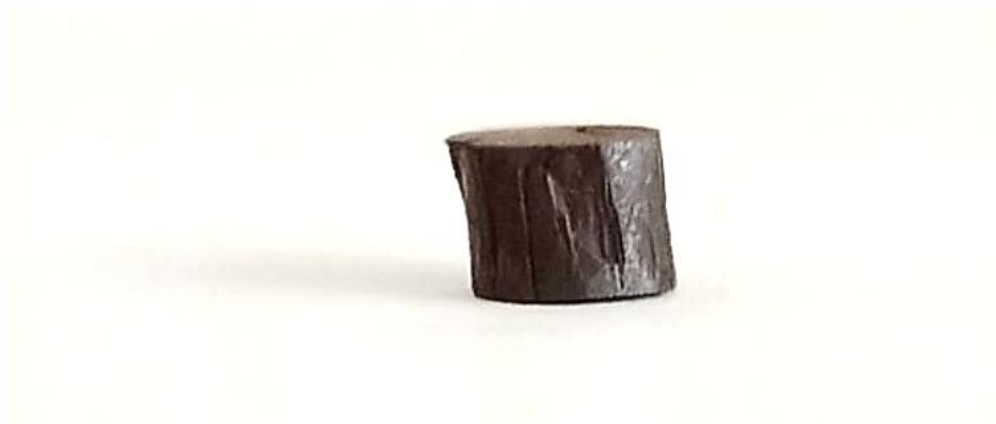
Figure 5-2 Representative image of the obtained pellet from SrM_LTSSR_R10/45 powders after M.A. compaction at 80°C and 4 GPa.
