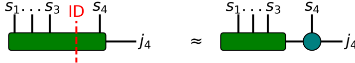
Figure 3.3.9. Third application of ID, separating index s_4 and recording (s_4, s_5, s_6) .
