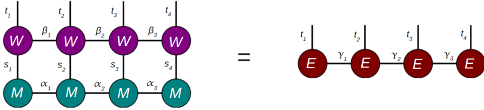
Figure 3.2.3. Graphical representation of the contraction between two sets of tensors, M and W , in Penrose notation. Connecting legs indicate contracted indices, while free legs represent uncontracted indices, making the structure of the computation immediately clear.
