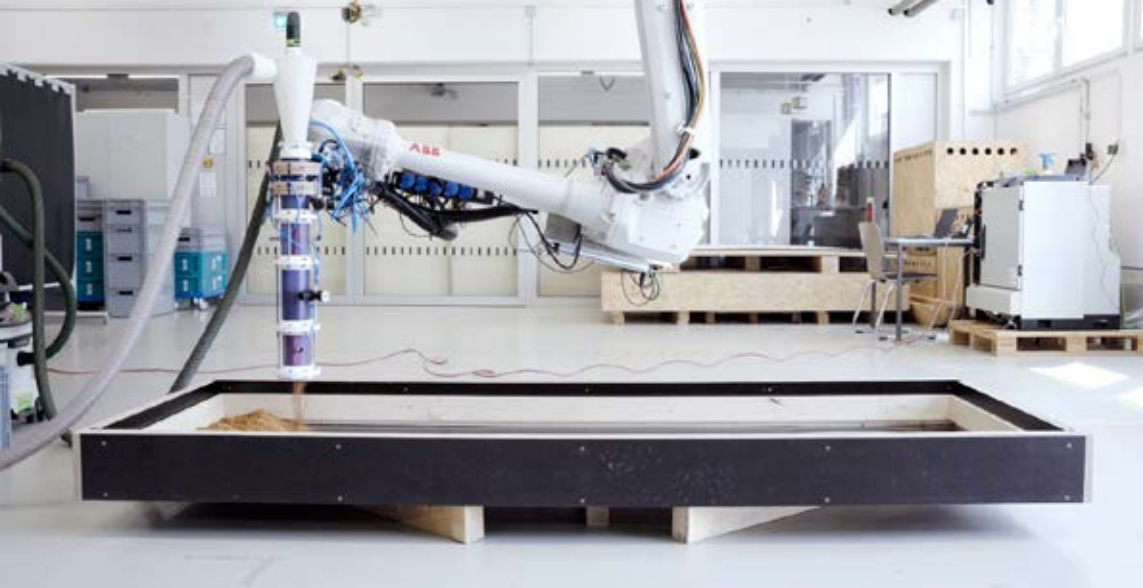
Fig. 11: AM process with mycelium substrates, combining sawdust-based and hemp-based mixtures for acoustic and structural customization.
