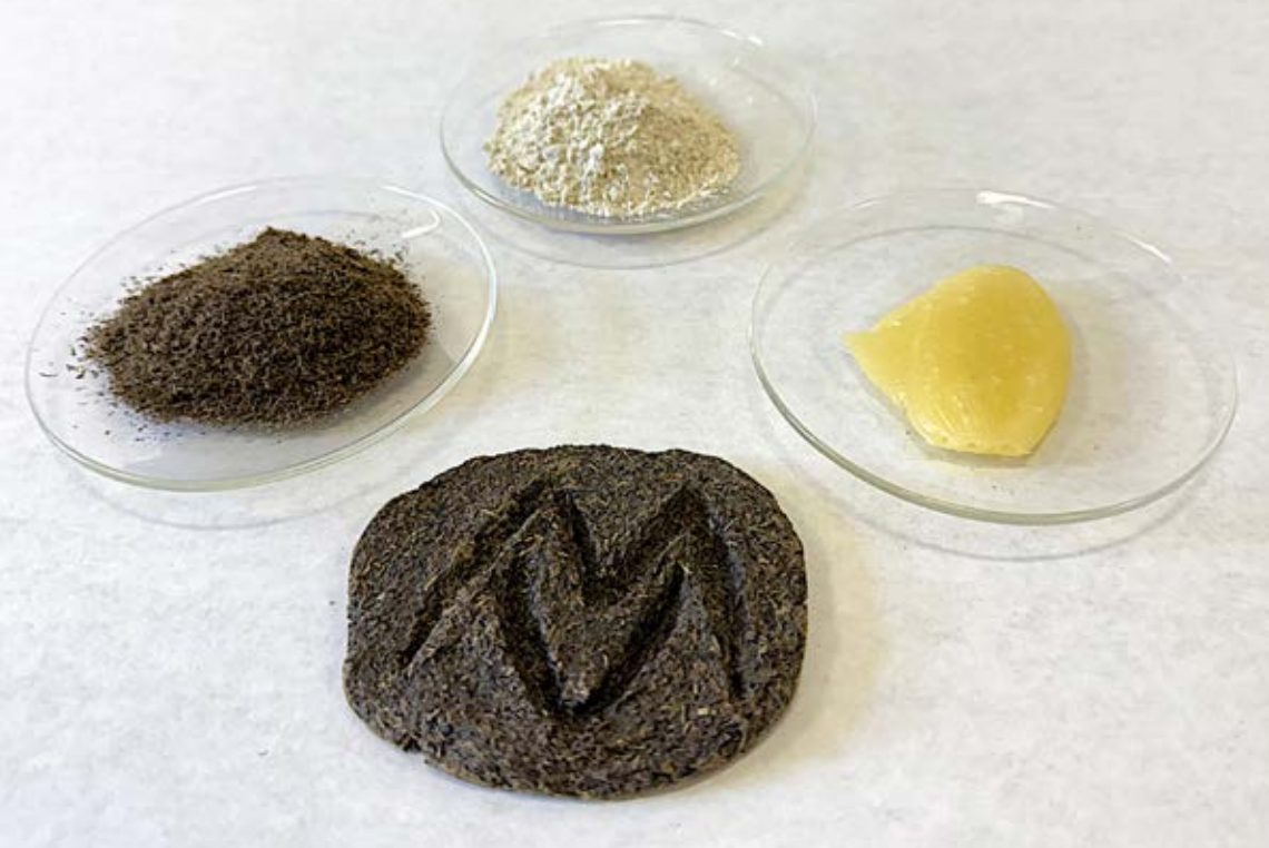
Fig. 3: Cured samples of the 3D biopaste (middle) and base raw materials
