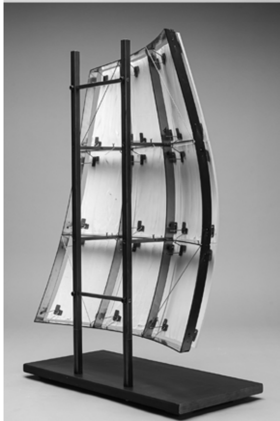
Fig. 7: Photos of the 1:10 scale facade prototype composed of 3 \times 3 panels fabricated with our flexible mold. finished panel with smooth outer surface (bottom left) and textured inner surface (bottom right).
