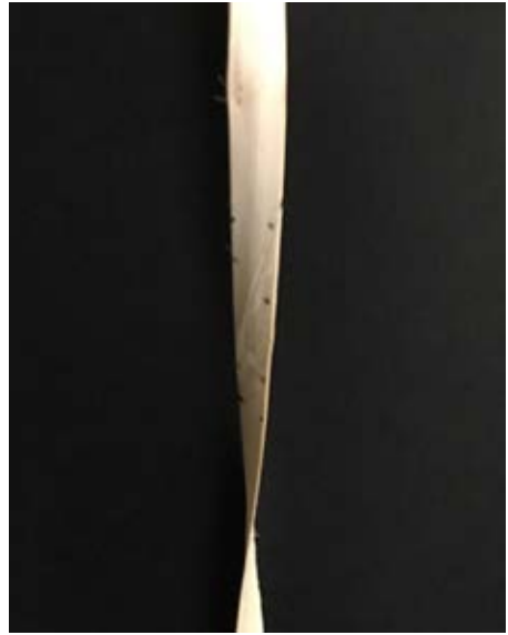
Fig. 2: Continuous wood monofilament made from willow rods ( Salix americana ). The 1–2 m rods are split, homogenized to a standardized rectangular cross-section, and joined through angled scarf joints with adhesive bonding.
