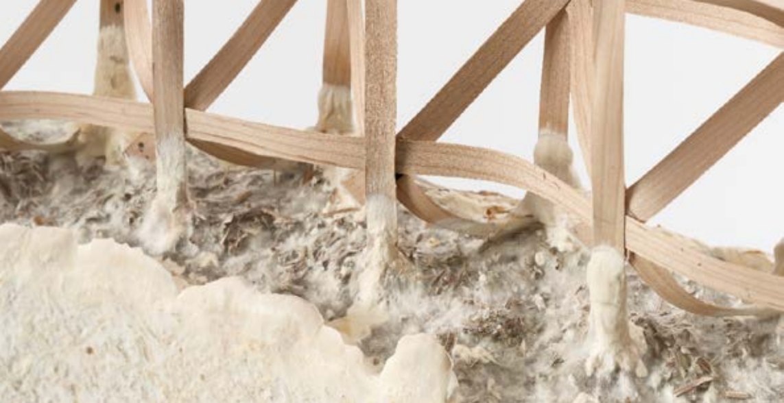
Fig. 10: Veneer lattices used as structural reinforcement for mycelium composites.
