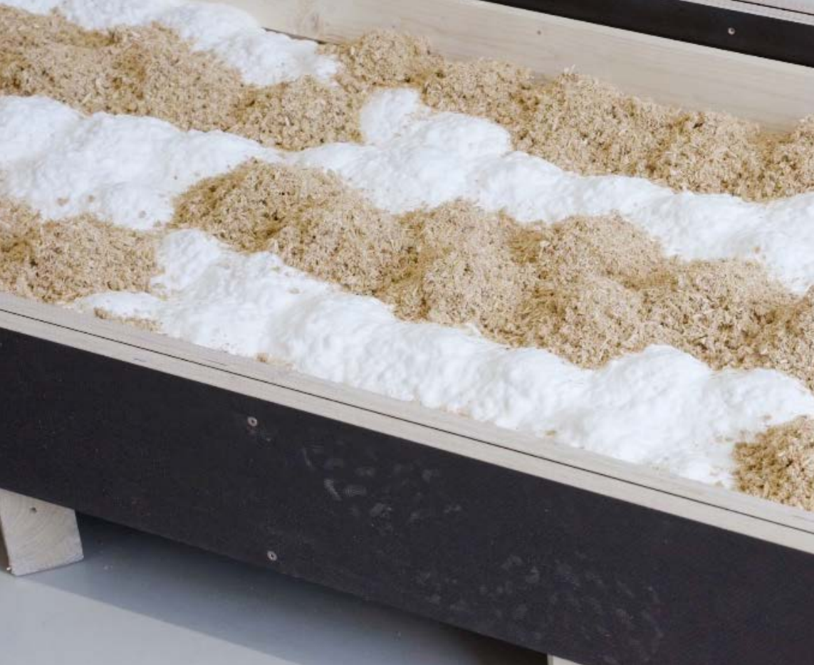
Fig. 12: AM process with mycelium substrates, combining sawdust-based and hemp-based mixtures for acoustic and structural customization.
