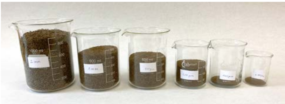
Fig. 4: Fractions of a refined Magaverde biofiber sample
