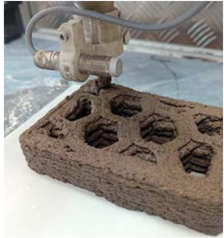
Fig. 6: Adapted clay 3D printing system during the fabrication of a honeycomb demonstrator made from Magaverde biofiber paste.
