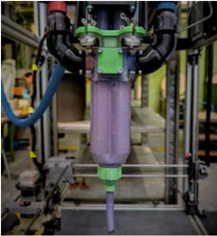
Fig. 5: Twin-screw extruder setup during testing of blending of two dyed pastes (blue and red)
