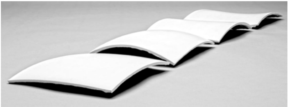
Fig. 4: From left to right, manually fabricated gypsum panels TP1 ( K > 0 ), TP2 ( K >> 0 ), TP4 ( K < 0 and K > 0 ), and TP3 ( K < 0 ).
