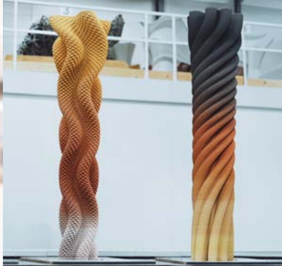
Fig. 5: Printed concrete columns
