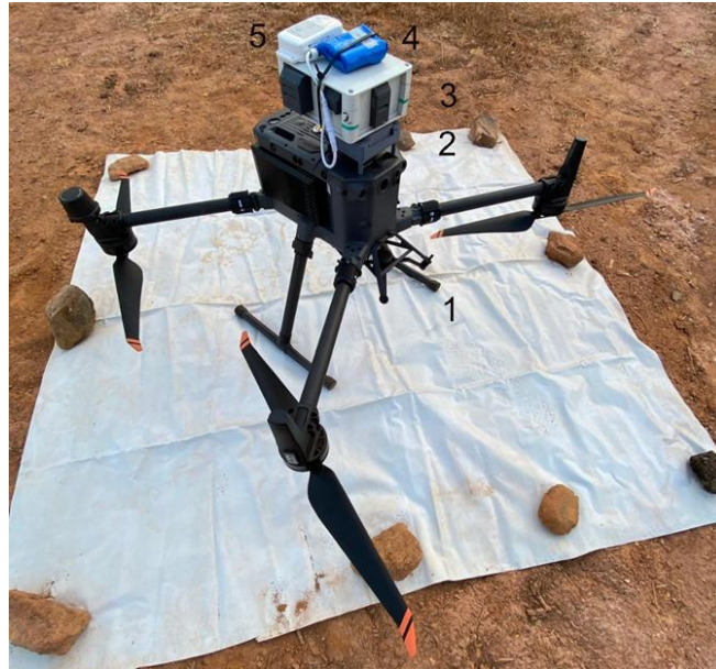
Figure 4. The UAV-based system and its parts: 1. the UAV; 2. the 3D-printed support; 3. the MSP; 4. the power bank; 5. the Temperature/RH Data Logger.
