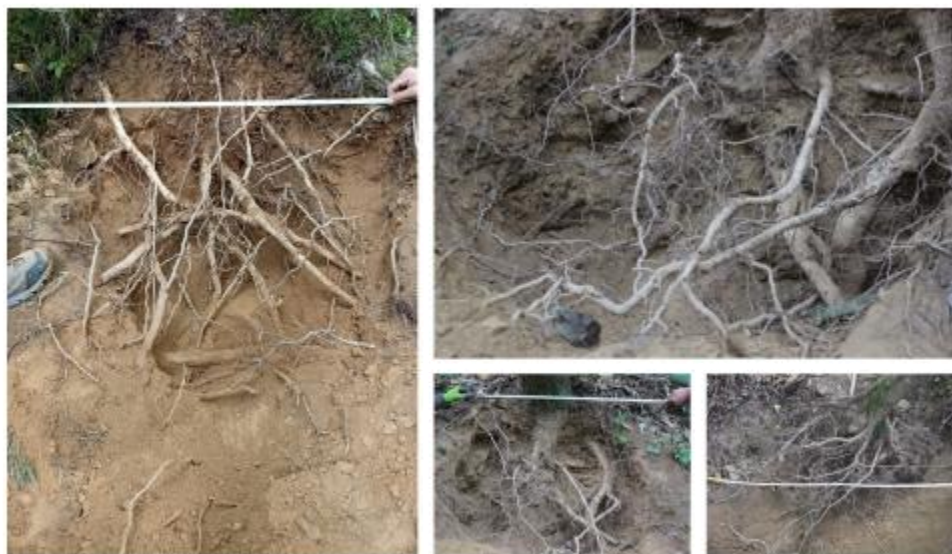
Figure 7: Root system field survey in AdS1-SWBE restored landslide, for Ar and RAR value detection, for the representative tree species: Alnus incana , Castanea sativa and Ostrya carpinifolia .
