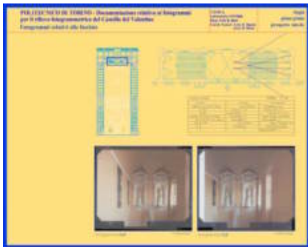
Figure 1. Valentino's Castle Turin. An Example of stereoscopic couple card obtain in different periods. Central prospect towards the backyard (up);stereoscopic of the open gallery of the stair; stereocouple central body .
