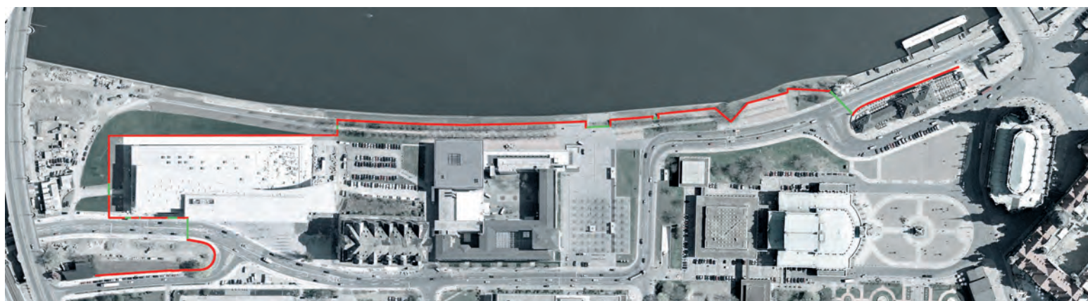
Central part of the planned protection line for the 'Historical old town' and 'Wilsdruffer Vorstadt' city districts, as from May 2005 with stationary (red) and mobile (green) elements (Peter Kulka Architektur Dresden GmbH)
